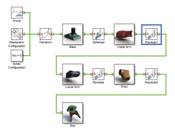
Joint blocks are assortments of joint primitives, basic yet complete joints of various kinds you cannot decompose any further—at least without losing behavior such as the rotational-translational coupling of the lead screw joint. Joint primitives range in number from zero in the Weld Joint block to six in the Bushing Joint block. There are five joint primitives:
